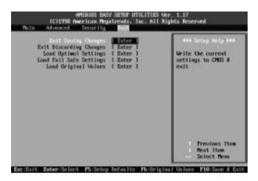
Exit Saving Changes allows you to write the current settings to CMOS and exit.
