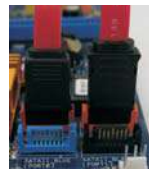
Connect the SATA data cables to both red SATAII connector (SATAII_RED (PORT2)) and orange SATAII connector (SATAII_ORANGE (PORT3))
