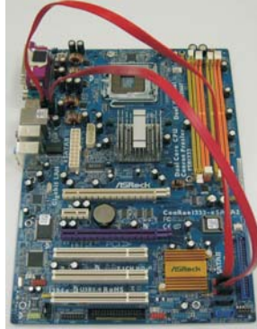
Connect the SATA data cables to both red eSATAII connector (eSATAII_BOTTOM) and orange eSATAII connector (eSATAII_TOP)
