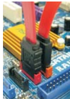
Connect the SATA data cables to both red SATAII connector (SATAII_RED (PORT2)) and orange SATAII connector (SATAII_ORANGE (PORT3))
