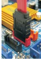
Connect the SATA data cable to the red SATAII connector (SATAII_RED (PORT2))
