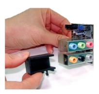
2. Align the module's plugs above the mounting holes then insert the plugs from the top through to the bottom of the system board. While at it, the I4-pin connector at the solder side of the module must also insert into the Karajan audio connector at location J7 of the system board. Make sure the plugs snap firmly out the bottom of the board.
