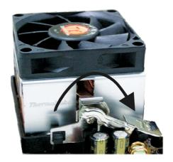
6. Connect the CPU fan's cable connector to the CPU fan connector on the system board.
