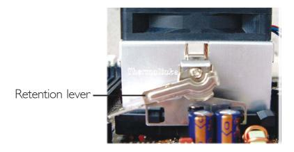
5. Move the retention lever to its opposite side then push it down to lock the fan and heat sink assembly to the retention module base.
