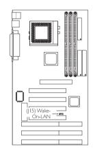
card and the other end to location JI5 on the system board. The network will detect Magic Packet and assert a wakeup signal to power-up the system. Refer to the add-in card's manual for details. Note: Your LAN card must support the remote wake up function.
