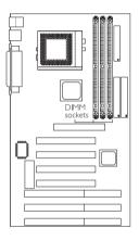
The system board is equipped with three I68-pin DIMM (Dual In-line Memory Module) sockets that support x64/x72 PC SDRAM DIMM, 3.3V. PC SDRAM (Synchronous Dynamic Random Access Memory) uses a fast memory interface technology that includes using the clock on the chip to synchronize with the CPU clock so that the timing of the memory chips and the timing of the CPU are synchronized. This saves time during transmission of data, subsequently increasing system performance.
