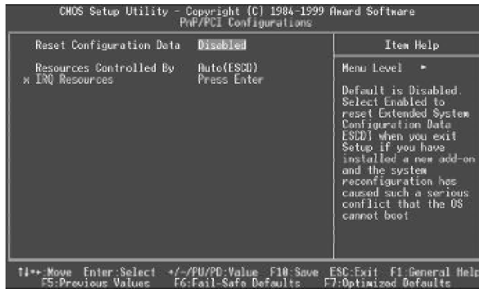
Figure-7 PNP/PCI Configuration Setup Menu
