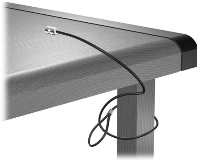
Figure C-3 Securing the Cable to a Fixed Object
