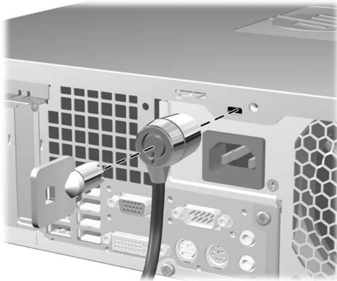
Figure C-1 Installing a Cable Lock
