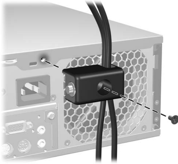
Figure C-5 Attaching the Lock to the Chassis
