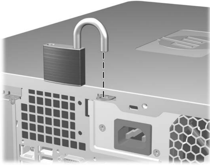
Figure C-2 Installing a Padlock
