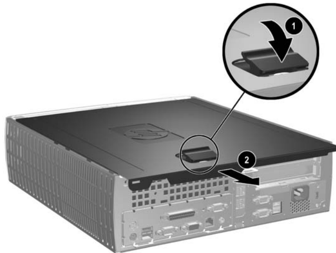
Removing the Computer Access Panel
