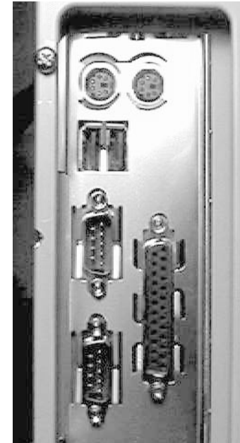
I/O connector's aligned with openings
