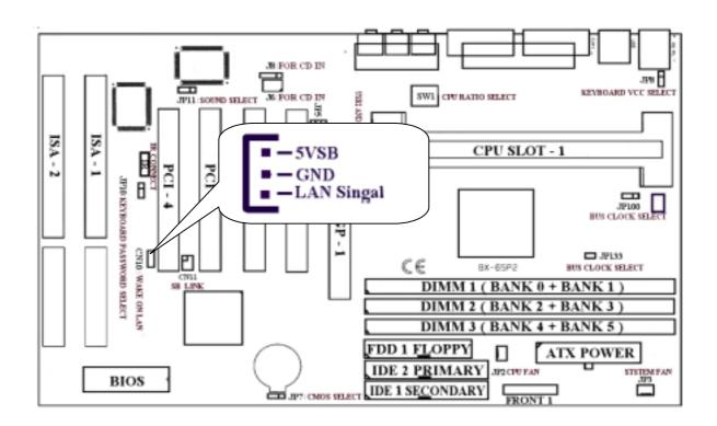
N11: SB\_LINK Connect (for PCI BUS Sound Cards . Sush As Creative Labs EMU 8088 Sound CHIP)
