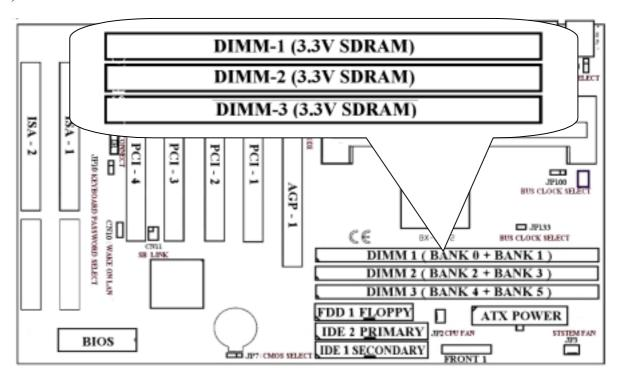
( 2 ) The Supports Different Type Of Settings For The System Memory . There Is No Jumper Nor Connect Needed For Memory Configuration . Following Figures Provides All Possible Memory Cominations .
