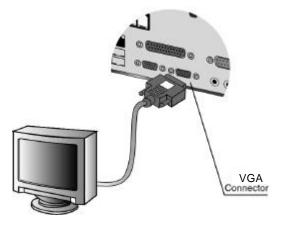
3. Connect a computer VGA monitor to the VGA connector.
