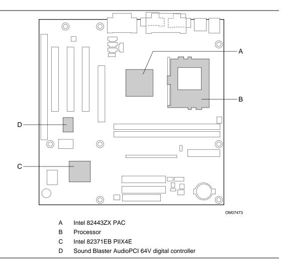
Figure 13. Thermally-sensitive Components
