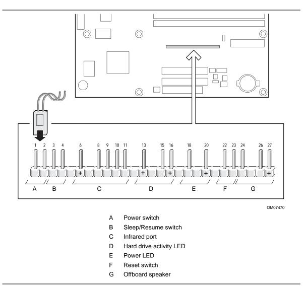
Figure 8. Front Panel Connector
