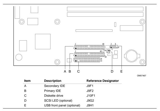
Figure 5. Peripheral Interface and Indicator Connectors
