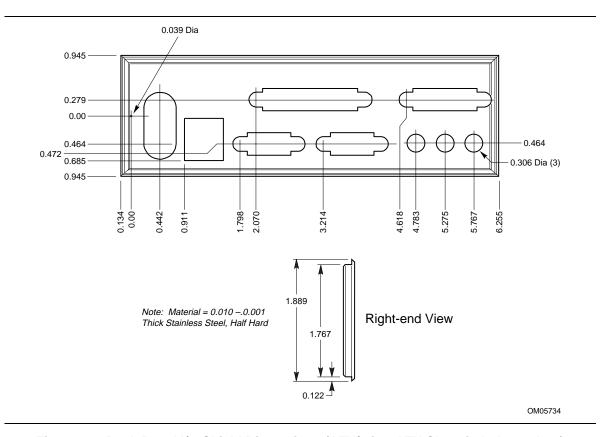
Figure 12. Back Panel I/O Shield Dimensions (ATX/microATX Chassis-Independent)
