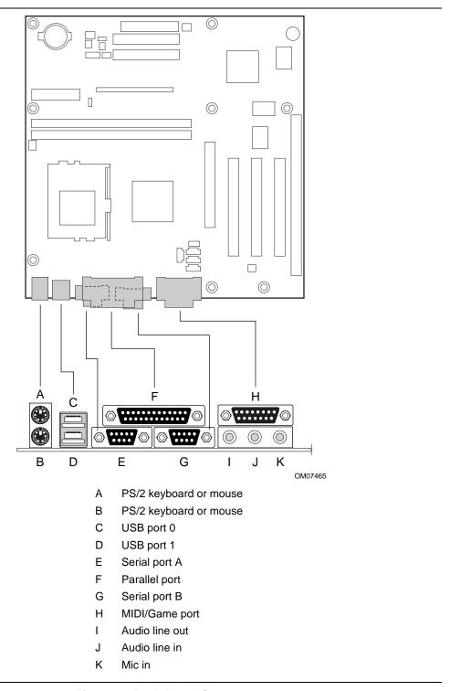
Figure 3. Back Panel Connectors
