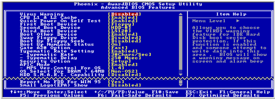
Figure 4-5. Advanced BIOS Features Setup Screen
