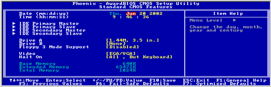
Figure 4-3. Standard CMOS Setup Screen Shot
