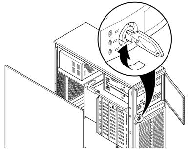
Figure 9-1. Security Door and Side Panel Chassis Lock
