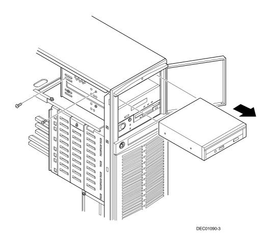
Figure 11-3. Removing and Replacing the CD-ROM Drive
