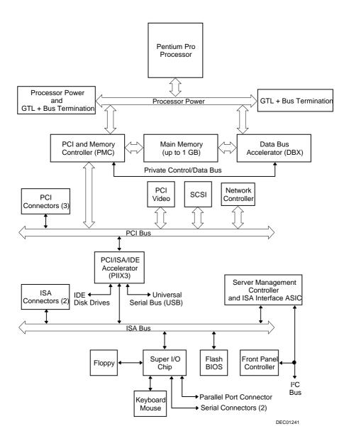
Figure E-1 Main Logic Board Block Diagram
