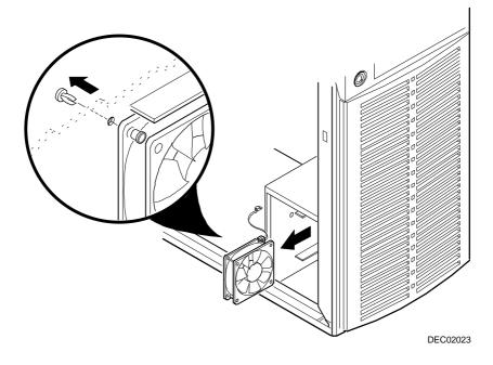
Figure 11-5. Removing and Replacing the Lower Cooling Fan
