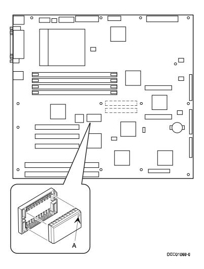
Figure 5-3. Installing a Video Memory Expansion Chip
