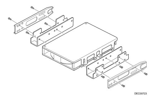
Figure 6-2. Installing Expansion Brackets
