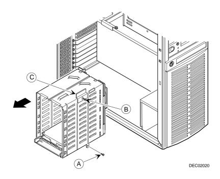
Figure 11-4. Removing and Replacing the Drive Bay Cooling Fan
