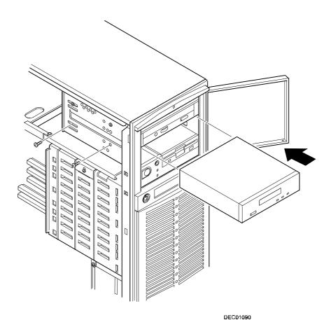
Figure 6-1. Installing a 5<sup>1</sup>/<sub>4</sub>-Inch Device into the Front Access Drive Bay
