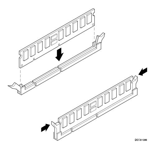
Figure 5-2. Installing a DIMM
