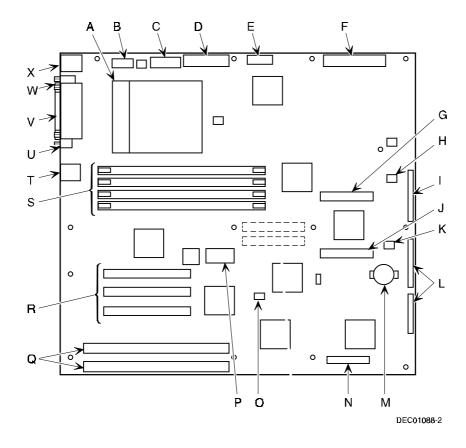
Figure 3-6. Main Logic Board Components and Connectors
