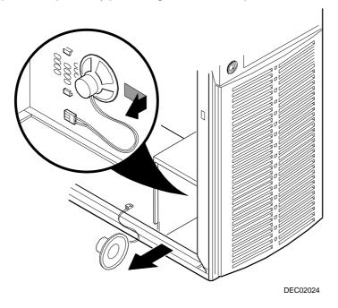
Figure 11-6. Removing and Replacing the Speaker
