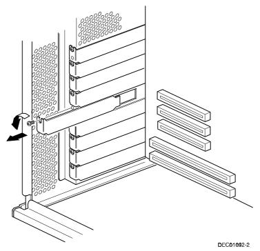
Figure 7-3. Removing a Metal Filler Plate
