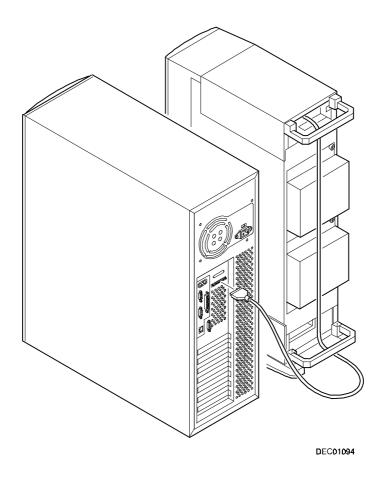
Figure 6-5. Connecting an External SCSI Storage Box
