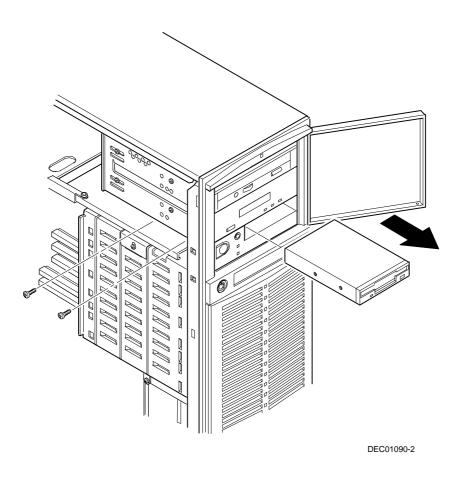
Figure 11-2. Removing and Replacing the Diskette Drive
