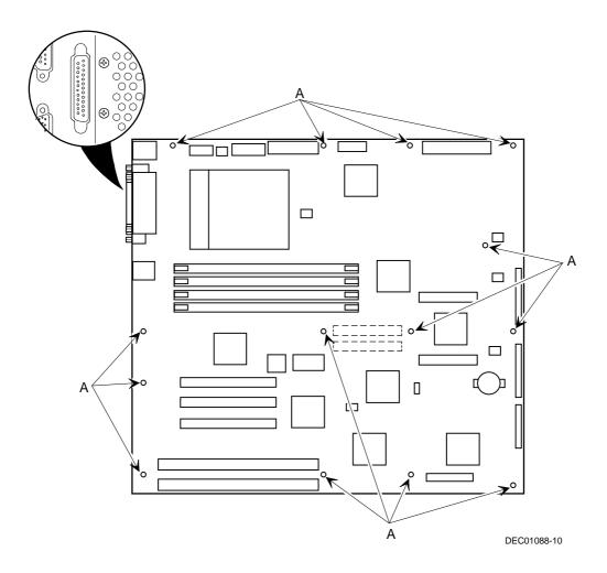
Figure 11-8. Removing and Replacing the Main Logic Board
