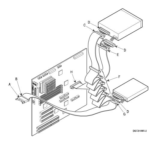
Figure 8-1. Single Channel SCSI Configuration
