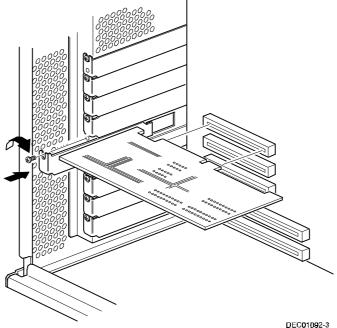
Figure 7-5. Installing a PCI Expansion Board
