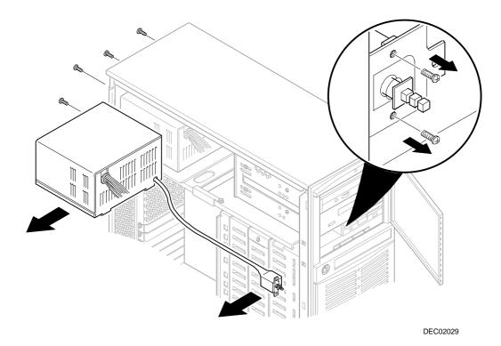
Figure 11-1. Removing and Replacing the Power Supply and Control Assembly
