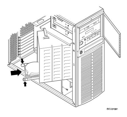
Figure 6-4. Installing a 3<sup>1</sup>/<sub>2</sub>-Inch Device Into the Internal Drive Bay
