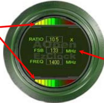
On the left circle area shows Ratio, FSB and frequency information about CPU. When the values are set to factory default, the light on the top and bottom of the circle will show green and it will vary as you change these CPU settings.
