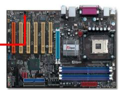
**Note:** Though some of the latest versions of Windows support "Digital Audio" through IDE bus. However, in order to use Open Jukebox player, which is driven under BIOS, it is a **MUST** to insert audio cable to CD-IN connector on the motherboard.
