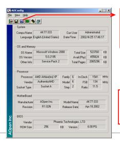
The system page shows the detail information of the motherboard, the operating system, the processor, and BIOS version.
