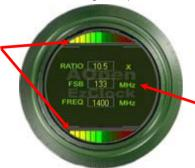
On the left circle area shows Ratio, FSB and frequency information about CPU. When the values are set to factory default, the light on the top and bottom of the circle will show green and it will vary as you change these CPU settings.
