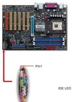
The pins of Front Panel Connector are painted in different colors with their respective functions. Please attach the power LED, speaker, power and reset switch connectors to the corresponding pins matched in same colors. If you enable "Suspend Mode" item in BIOS Setup, the ACPI & Power LED will keep flashing while the system is in suspend mode.
