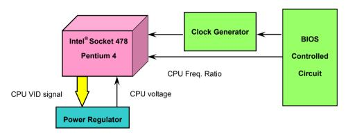
(Automatically generates CPU voltage)
