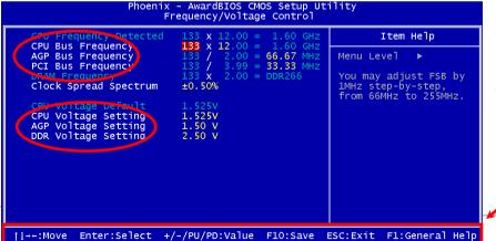
"+", "-", "PqUp" or "PqDn" keys, you can adjust the frequency values of CPU Bus, PCI Bus and DRAM.
