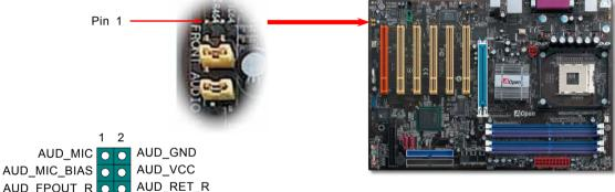
**Note:** Please remove the jumper cap from the Front Panel Audio Connector before you connect the cable. Do not remove this yellow jumper cap if housing without an audio port on the front panel.
