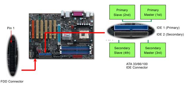
IDE1 is also known as the primary channel, IDE2 is known as the secondary channel. Each channel supports two IDE devices that make a total of four devices. In order to work together, the two devices on each channel must be set differently to **Master** and **Slave** mode. Either one can be the hard disk or the CDROM. The setting as master or slave mode depends on the jumper on your IDE device, so please refer to your hard disk and CDROM manual accordingly.
