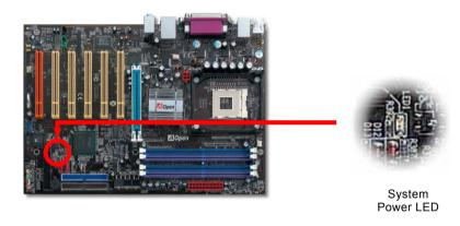
Warning: Do not install or remove the DIMM module or others devices when the STBY LED lights on.
