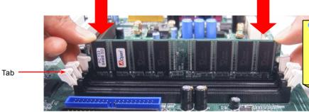
Note: The tabs of the DIMM slot will close-up to hold the DIMM in place when the DIMM touches the slot's bottom.
