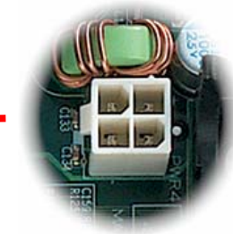
4-Pin 12V ATX Power Connector
