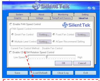
**CD-ROM Rotation Speed Control**: by enabling the CD-ROM Rotation Speed Control, you can adjust the rotation speed of your CD-ROM. When you set the speed to high level, the CD-ROM will work at its fastest speed and it will run at basic required speed while you set the value to low speed.
