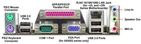
PS/2 Keyboard: For standard keyboard, which use a PS/2 plug.
