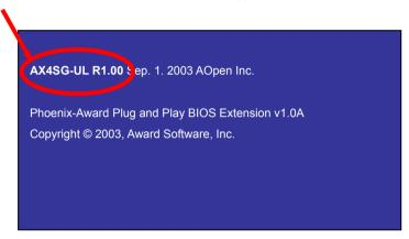
AX4SG-UL is model name of motherboard; R1.00 is BIOS version.
