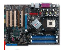
The pins of Front Panel Connector are painted in different colors with their respective functions. Please attach the power LED, speaker, power and reset switch connectors to the corresponding pins matched in same colors. If you enable "Suspend Mode" item in BIOS Setup, the ACPI & Power LED will keep flashing or high light while the system is in suspend mode.
