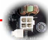
4-Pin 12V ATX Power Connector
