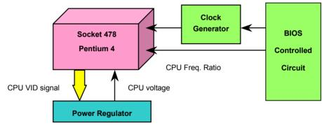
(Automatically generates CPU voltage)
