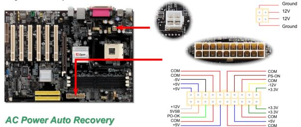
A traditional ATX system should remain at power off stage when AC power resumes from power failure. This design is inconvenient for a network server or workstation, without an UPS, that needs to keep power-on. This motherboard implements an AC Power Auto Recovery function to solve this problem.
