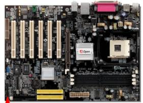
Attach the power LED, Keylock, speaker, power and reset switch connectors to the corresponding pins. If you enable "Suspend Mode" item in BIOS Setup, the ACPI & Power LED will keep flashing while the system is in suspend mode.
