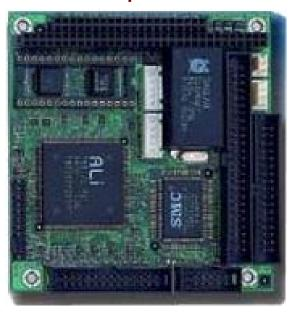
The AX10402 is a PC/104 plug-in CPU module using 80386SX 40-MHz. Its 6-layer printed circuit board combines features with noise-tolerant and low power consumption. CMOS technology applied on the board makes AX10402 withstand and adapt harsh industrial environments very well.
