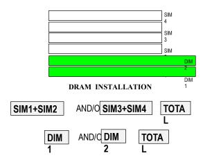
The 72-pin group includes four SIMMs; each SIMM can be 4, 8,16, or 32MB in size. The 168-pin group includes two DIMMs; each DIMM can be 8, 16, 32, or 64MB in size. Please use the RAM modules of the same size in the group. Auto-banking memory features are supported for SIMMs or DIMMs.
