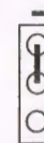
Some jumpers are oriented vertically; if the pin position needs to be shown, Pin 1 is marked.
