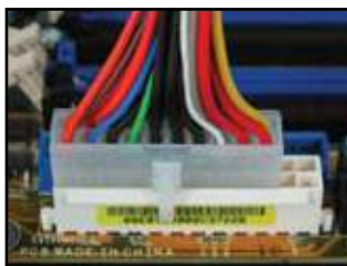
20-pin power connector (on the 24-pin female counterpart)
