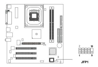
JFP1 Switch/LED Front Panel Electrical Connection
