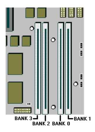
SIMMs must be fitted in pairs and the pair must be identical. The system does not require Parity checking (36-bit) SIMMs. Conventional 32-bit SIMMs with a refresh rate of 70ns is the specification. The newer Extended Data Output (EDO) type SIMMs are supported and will give enhanced performance.
