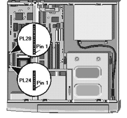
This range of pins is not exactly for jumpers, but is used to connect various features around the system case to the motherboard.
