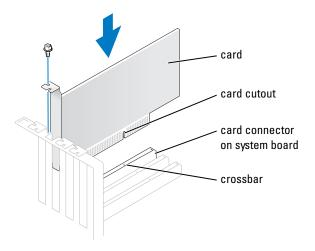
Ensure that the card is fully seated and that its bracket is within the card slot.
