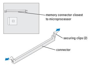
**9** Align the notch on the bottom of the module with the crossbar in the connector.
