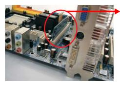
PCIE Switch card on PCIE2/PCIE SWITCH slot
