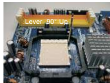
STEP 1: Lift Up The Socket Lever
