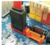
Connect the SATA data cable to the red SATAII connector (SATAII_RED (PORT 2.1))
