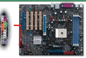
Attach the power LED, speaker, and reset switch connectors to the corresponding pins. If you enable "Suspend Mode" item in BIOS Setup, the ACPI & Power LED will keep flashing while the system is in suspend mode.
