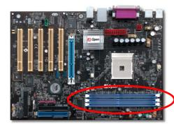
Note: According to the standard DDR400 specification from JEDEC (Joint Electron Device Engineering Council), it is regulated that DDR400 supports only 2x DIMM on the memory module for a maximum 2GB capacity, and DDR333 supports up to 3x DIMM for a maximum of 3GB capacity. Please be noted that K8T800 series motherboards follow this standard specification on memory as well.
