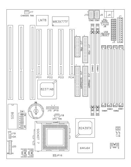
Figure 1: Layout of the AI5TT Motherboard
