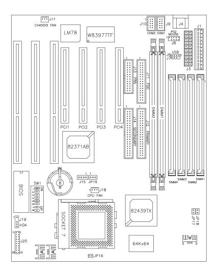
Figure 2: Jumper Location of the AI5TT
