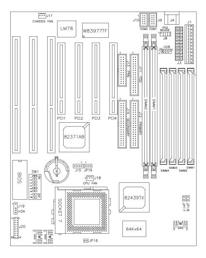
Figure 3: Connector Locations of the AI5TT
