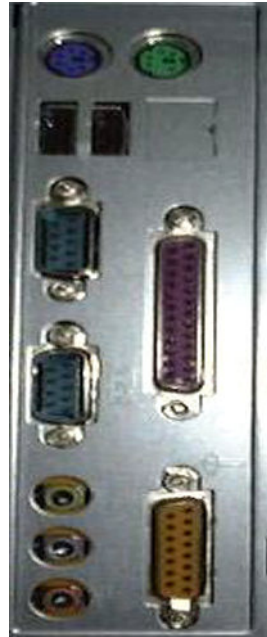
I/O connectors aligned with openings
