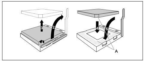
Pull the lever in the direction of the arrow (1) and lift it as far as it will go (2).
