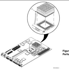
Figure 3 - 13 Installing a Higher Performance CPU
