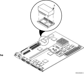
Figure 3 - 15 Replacing the Computer Battery
