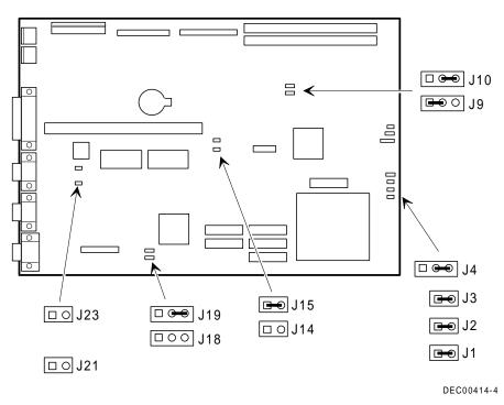
Figure 3 - 6 Main Logic Board Jumper Locations
