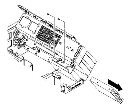
Figure 3 - 9 Removing the 3<sup>1</sup>/<sub>2</sub>-Inch Diskette Drive
