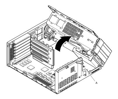
Figure 3 - 8 Opening the Device Bay & Power Supply Subassembly
