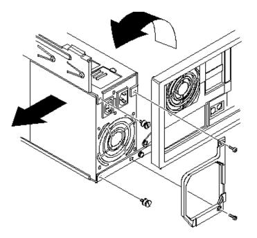
Figure 3 - 11 Removing the on Power Supply
