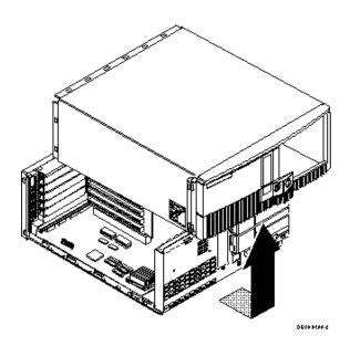
Figure 3 - 3 Removing the Cover
