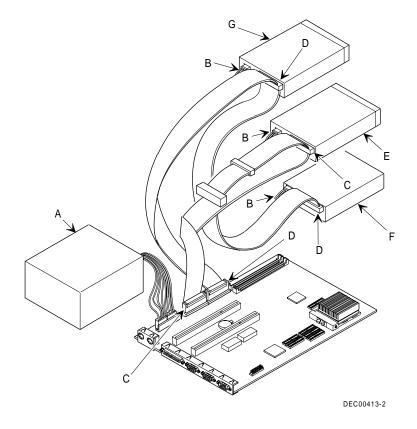
Figure 3 - 16 Diskette/IDE Drive Data Cable Connections
