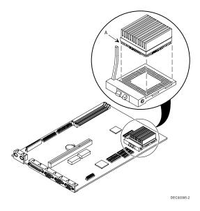
Figure 3 - 14 Installing a Higher Performance
