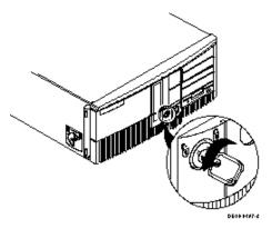
Figure 3 - 1 Unlocking the Cover
