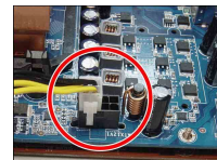
Plugged from a 4-pin ATX12V power.
