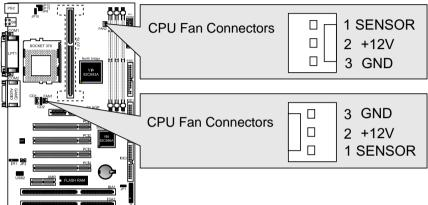
Note: The CPU and motherboard will overheat if there is no airflow across the CPU and onboard heatsink. Damage may occur to the motherboard and the CPU fan if these pins are incorrectly used. These are not jumpers, do not place jumper caps over these pins.
