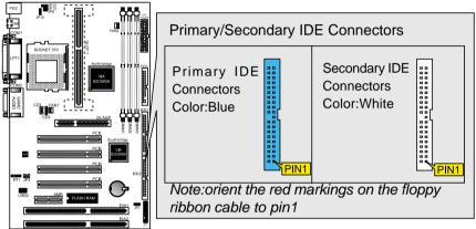
Note: Ultra DMA/66 IDE devices must use an 80-wire IDE cable or else devices will automatically be limited to Ultra DMA/33 mode.
