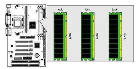
orientation shown. The DIMM must be 3.3V for this motherboard.
