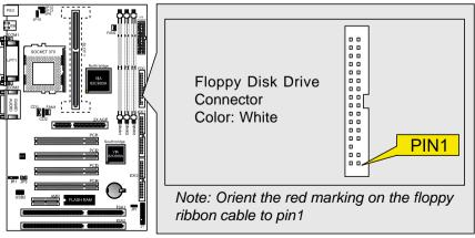
You can attach up to two floppy drives to the motherboard. After connecting the single end to the board, connect the two plugs on the other end to the floppy drives. The drive A: should be connected on the end and the drive B: in the middle.
