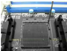
STEP 1: Lift Up The Socket Lever
