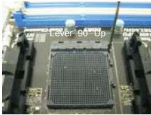
STEP 1: Lift Up The Socket Lever
