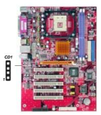
When you first start up your system, the BIOS should automatically detect your CD-ROM/DVD drive. If it doesn't, enter the Setup Utility and configure the CD-ROM/DVD drive that you have installed. On the motherboard, locate the 4-pin header **CD1**.
