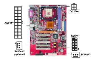
Connect the power connector from the power supply to the **ATXPW1** connector on the motherboard. The **CPUPW** is a +12V connector for CPU Vcore power.
