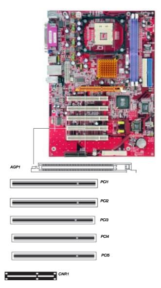
Follow the steps below to install an AGP/CNR/PCI expansion card.
