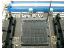
STEP 1: Lift Up The Socket Lever
