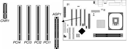
Follow the steps below to install an AGP/CNR/PCI expansion card.
