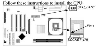
1. Unhook the locking lever of the CPU socket. Pull the locking lever away from the socket and raising it to the upright position.
