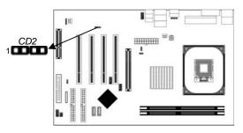
When you first start up your system, the BIOS should automatically detect your CD-ROM/DVD drive. If it doesn't, enter the Setup Utility and configure the CD-ROM/DVD drive that you have installed. On the motherboard, locate the 4-pin connector **CD2**.
