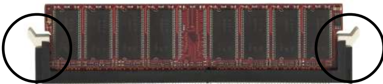
Figure 9 - DIMM module clip after installation
