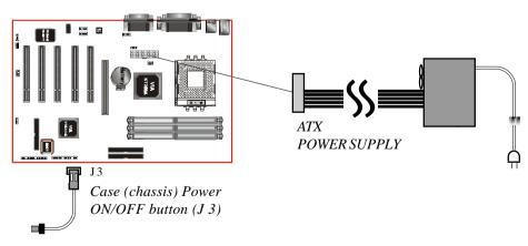
Figure 4: Simple ATX Power ON/OFF Controller
