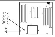
JP11, JP12, JP13, JP14, JP16 - Power Selection for the CPU Core Voltage, Bus Section and Bus Voltage
