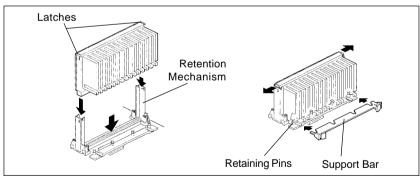
Slide the top heatsink support bar onto the retaining pins of the support's base as shown in figure.
