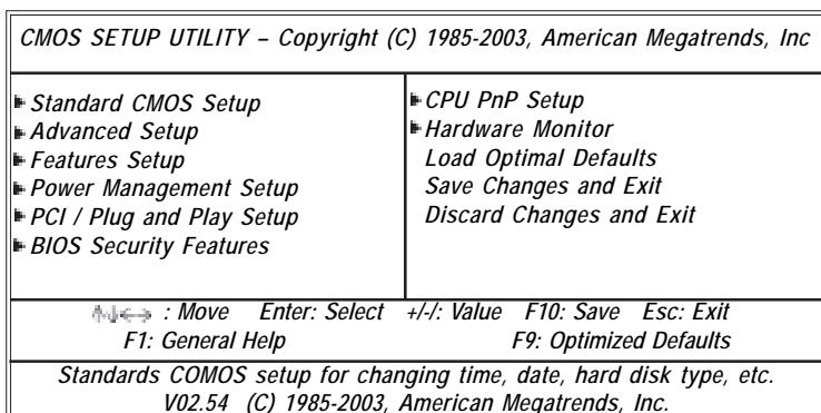
You can use cursor arrow keys to highlight anyone of options on the main menu page. Press **Enter** to select the highlighted option. Press the **Escape** key to leave the setup utility. Press +/- to modify the selected field's values.
