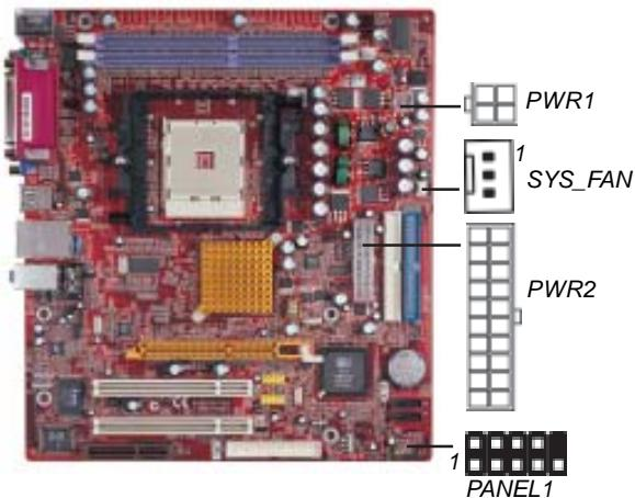
Connect the power connector from the power supply to the **PWR2** connector on the motherboard. The **PWR1** is a +12V connector for CPU Vcore power.
