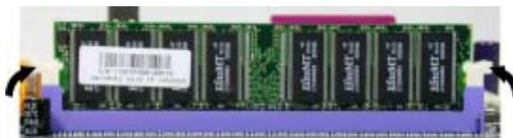
4. Install any remaining DIMM modules.
