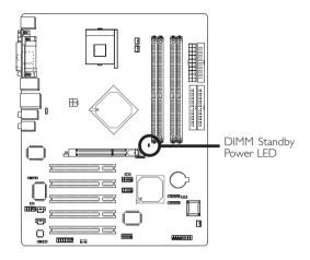
This DIMM Standby Power LED will turn red when the system's power is on or when it is in the Suspend state (Power On Suspend or Suspend to RAM). It will not light when the system is in the Soft-Off state.
