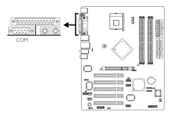
The system board is equipped with an onboard serial port (Teal/Turquoise) at location CN4 of the system board. It is a RS-232C asynchronous communication port with 16C550A-compatible UART that can be used with a modem, serial printer, remote display terminal or other serial devices.
