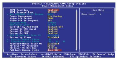
The screen above list all the fields available in the Power Management Setup submenu, for ease of reference in this manual. In the actual CMOS setup, you have to use the scroll bar to view the fields. The settings on the screen are for reference only. Your version may not be identical to this one.
