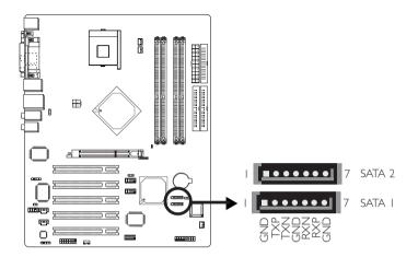
The system board is equipped with 2 SATA connectors at locations J16 (SATA 2) and J17 (SATA 1) for connecting serial ATA devices. Connect one end of the SATA cable to a SATA connector and the other end to your serial ATA device.
