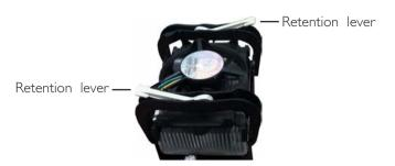
4. Move the retention levers to their opposite directions then push them down. This will secure the fan / heat sink and retention mechanism assembly to the retention module base.
