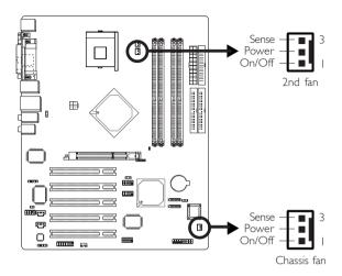
The chassis fan connector (J22) and 2nd fan connector (J14) are used to connect cooling fans. The cooling fans will provide adequate airflow throughout the chassis to prevent overheating the CPU and system board components. The system is capable of monitoring and controlling the speed of these cooling fans. These fans will automatically turn off once the system enters the Suspend mode.
