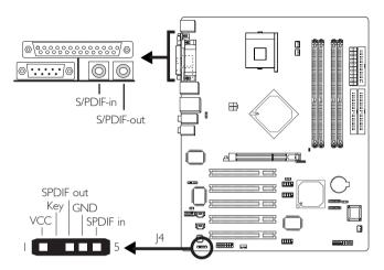
The system board is equipped with an onboard S/PDIF-in RCA jack (red) and a S/PDIF-out RCA jack (yellow) at locations CN5 and CN6 of the system board.
