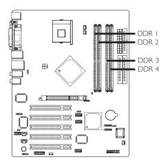
The system board supports DDR SDRAM DIMM. Double Data Rate SDRAM (DDR SDRAM) is a type of SDRAM that doubles the data rate through reading and writing at both the rising and falling edge of each clock. This effectively doubles the speed of operation therefore doubling the speed of data transfer.
