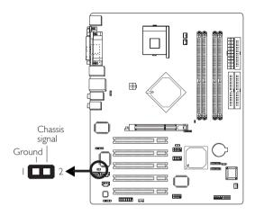
The system board supports the chassis intrusion detection function. To use this function, connect the chassis intrusion sensor cable from the chassis to J3. Whenever a chassis component has been removed, the sensor sends signal to J3 alerting you of a chassis intrusion event. To disable this function, place a jumper cap over J3.
