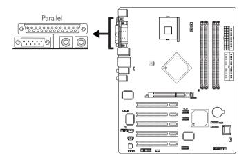
The system board has a standard parallel port (Burgundy) at location CN9 for interfacing your PC to a parallel printer. It supports SPP, ECP and EPP.
