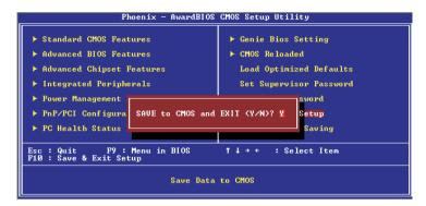
Type "Y" and press <Enter>. The modifications you have made will be written into the CMOS memory, and the system will reboot. You will once again see the initial diagnostics on the screen. If you wish to make additional changes to the setup, press <Ctrl> <Alt> <Esc> simultaneously or <Del> after memory testing is done.
