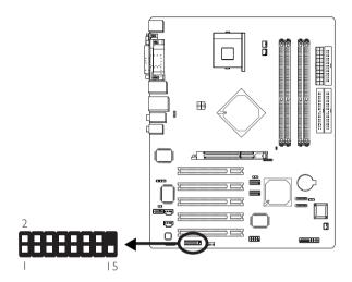
The system board is equipped with a 15-pin connector at location J7 for connecting an external game/MIDI port. The game port may be mounted on a card-edge bracket. Install the card-edge bracket to the system chassis then connect the game/MIDI port cable to connector J7. Make sure the colored stripe on the ribbon cable is aligned with pin 1 of connector J7.
