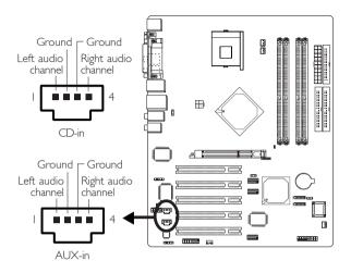
The CD-in (J5) and AUX-in (J6) connectors are used to receive audio from a CD-ROM drive, TV tuner or MPEG card.
