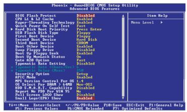
The screen above list all the fields available in the Advanced BIOS Features submenu, for ease of reference in this manual. In the actual CMOS setup, you have to use the scroll bar to view the fields. The settings on the screen are for reference only. Your version may not be identical to this one.
