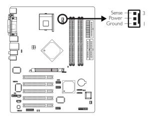
The CPU must be kept cool by using a fan with heatsink. Connect the CPU fan to the 3-pin fan connector at location JI3 of the system board. The system is capable of monitoring the speed of the CPU fan.
