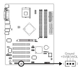
Your LAN card package should include a cable. Connect one end of the cable to the wakeup header on the card and the other end to location J8 on the system board. The network will detect Magic Packet and assert a wakeup signal to power-up the system. Refer to the add-in card's manual for details. Note: Your LAN card must support the remote wake up function.
