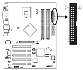
The system board is equipped with a shrouded floppy disk drive connector that supports two standard floppy disk drives. To prevent improper floppy cable installation, the shrouded floppy disk header has a keying mechanism. The 34-pin connector on the floppy cable can be placed into the header only if pin I of the connector is aligned with pin I of the header.
