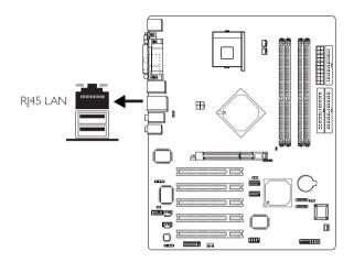
The system board is equipped with an onboard RJ45 fast-ethernet LAN port at location CN8 of the system board. It allows the system board to connect to a local area network by means of a network hub.
