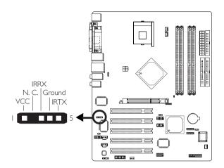
Connect your IrDA cable to connector J2 on the system board.
