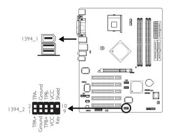
The system board is equipped with an onboard IEEE 1394 port at location CN7 of the system board.
