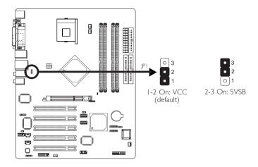
This jumper is used to select the power of the PS/2 keyboard and/or PS/2 mouse ports. Selecting 5VSB will allow you to use the Wake-On-PS/2 Keyboard/Mouse function.
