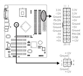
We recommend that you use a power supply that complies with the ATX12V Power Supply Design Guide Version I.I. An ATX12V power supply has a standard 20-pin ATX main power connector and a 4-pin +12V power connector that must be inserted onto CNII and CNIO connectors respectively.
