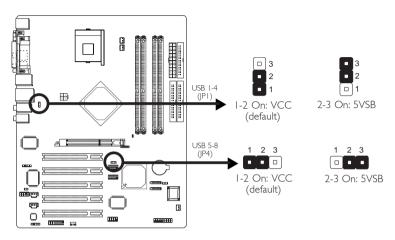
These jumpers are used to select the power of the USB ports. Selecting 5VSB will allow you to use the Wake-On-USB Keyboard function.
