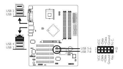
Four onboard USB 2.0/1.1 ports (Black) are at locations CN7 (USB 1-2) and CN8 (USB 3-4) of the system board.
