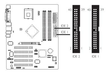
The system board is equipped with two shrouded PCI IDE headers that will interface four Enhanced IDE (Integrated Drive Electronics) disk drives. To prevent improper IDE cable installation, each shrouded PCI IDE header has a keying mechanism. The 40-pin connector on the IDE cable can be placed into the header only if pin I of the connector is aligned with pin I of the header.
