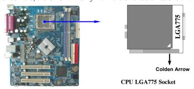
When you put the CPU into the LGA775 socket. No force require to insert of the CPU, then press the level to Locate position slightly without any extra force.
