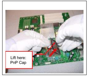
Note: After PnP cap removal, make sure socket load plate and contacts are free of foreign material; Refer to Overview Module for FM cleaning.
