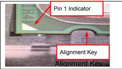
1. Lift processor package from shipping media by grasping the substrate edges ONLY.
