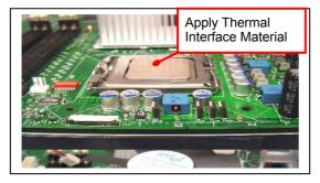
NOTE: Thermal Solutions that come with IntelR boxed processor use pre-applied thermal interface material and not grease.
