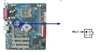
(3) USB Port connector: USB1, UL\_B (USB)
